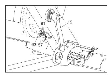
Next, turn the Left Crank Arm (19) until a Magnet (62) is aligned with the Reed Switch (57). Slide the Reed Switch slightly toward or away from the Magnet. Then, retighten the M4 x 16mm Screws (81).
