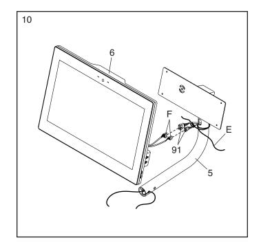
11. Tip: Avoid pinching the wires. If necessary, tilt the Console Bracket (26) upward to make this step easier. Attach the Console (6) to the Console Bracket with four M4 x 12mm Machine Screws (100); start all the Machine Screws, and then tighten them.
