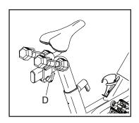
Note: The carriage handle (D) functions like a ratchet. Turn the carriage handle in the desired direction, pull it outward, turn it in the opposite direction, push it inward, and then turn it in the desired direction again. Repeat this process as many times as necessary.
