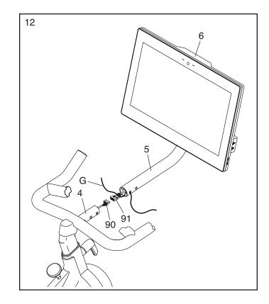
13. Tip: Avoid pinching the Wires (90, 91). Have the second person pull the console wires (F) but not the connectors out of the Console Mount (5) as you slide the Console Mount onto the Handlebar (4).
