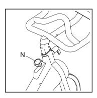
IMPORTANT: When the exercise bike is not in use, tighten the brake knob (N) completely.
